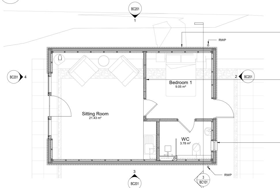
TIMBER CLADDED WALLS WITH SIPS INTERNAL STRUCTURE External wall comprising of horizontally installed (vertically installed on annex) weather treated
