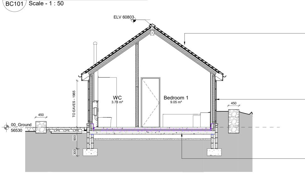
**ROOF STRUCTURE - VAULTED CEILINGS TO ANNEX**
